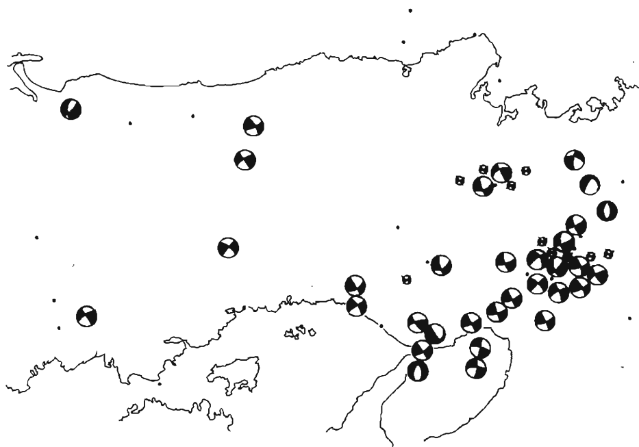
Fig. 24 Distribution of fault plane solutions of respective earthquakes in the whole region. Circles indicate fault plane solutions projected by Wullf's net and in respective circles black and white parts indicate dilatation and compression zones.
