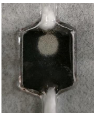
Figure 3.19 Photograph featuring the quartz reactor filled with Co 100 @ SiO 2 (500) after the PT-BRM activity test and XRD of the Co 100 @SiO 2 (500) after the PT-BRM activity test with the center of the irradiated spot (Blue) and the nonirradiated perimeter (Red).
