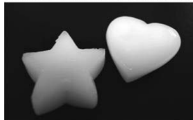
Figure 2. Chitin nanofiber-based hydrogels prepared at 35 wt% NaOH.
