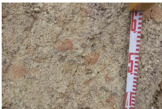
Fig. 42 Sliding surface material of white colored Kpfa (NGD-3).
