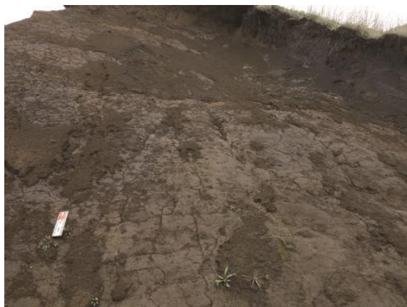
Fig. 16 A sliding surface in the mixed layer dominated by Br (KGC-4-1)
