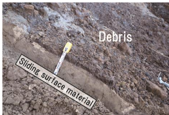
Fig. 14 A sliding surface formed in the mixed layer of tephra, which contained AT (KGC-2-2). The white layer to the left of the scale is AT.
