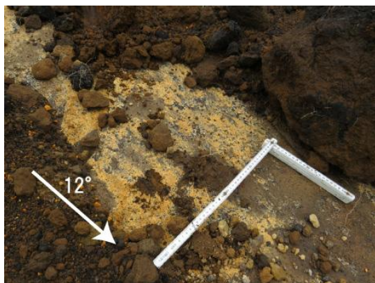
Fig. 23 An exposed sliding surface at the base of Kpfa (white), which occurs in patches on the underlying BILBr in AVL-1.
