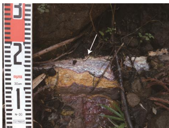
Fig. 20 Hydrothermal clay originated from lava in SWT-2. Colorful banding is observed.
