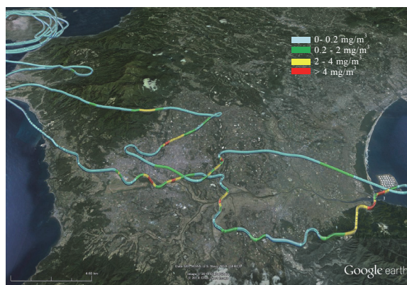
Fig.7 Flight path and ash concentration measured by DustMate on November 11, 2013.
