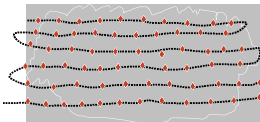
Fig. 1 Conceptual drawing of zig-zag measurement in a cross-section of plume. Red-color diamonds denote measurement points and dash line denotes flight path.
