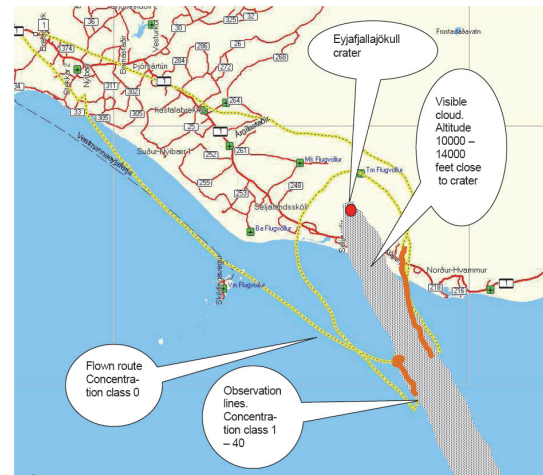
Fig. 2 Eyjafjallajökull volcano plume on May 11, 2010. Hatched area is plume and orange color lines are paths of airborne measurement by the University of Iceland group.
