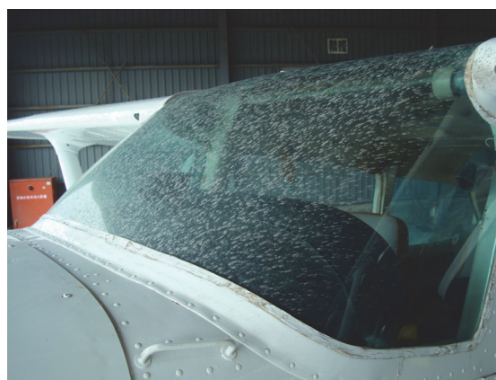
Photo 5 Front shield with ash deposit after flight through ash fallout.
