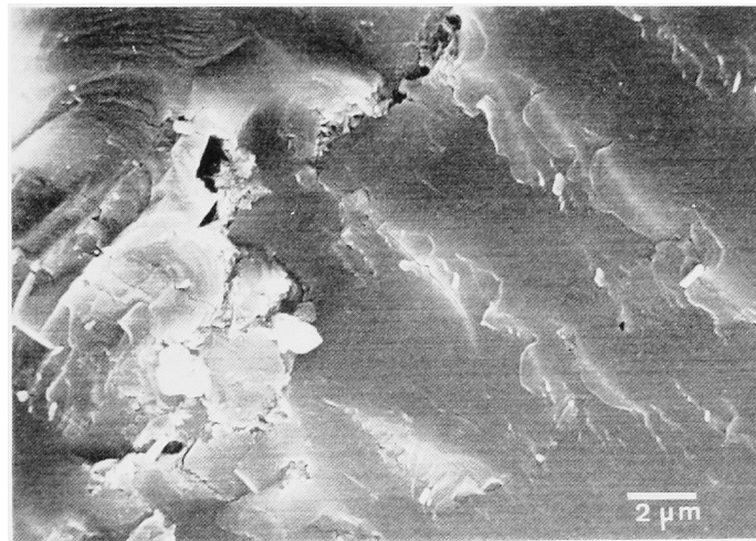
Fig. 8. Scanning electron micrograph showing concentric laminations of amorphous substances in the outer layer. Reduced from \times 5,000 .
