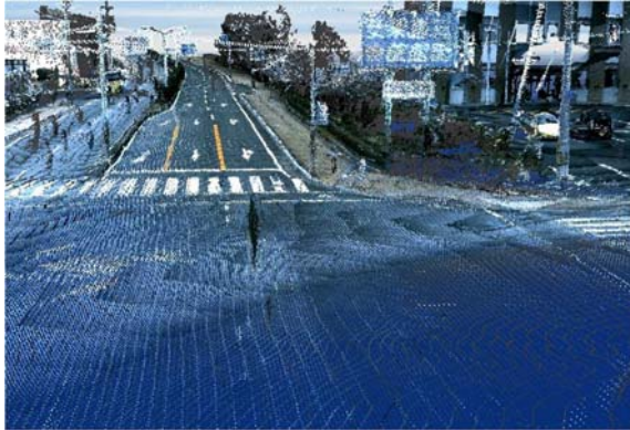
Fig. 9 Example of monitored results by the mobile mapping system at Oaki, Toba City
