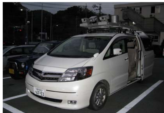
Fig. 8 Automobile with mobile mapping system
