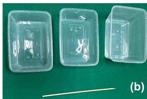
Fig. 3 Materials for assembling a FIT: (a) two sheets of A3-size transparent plastic document folder and two 70 cm-long orchid wires (already combined to form the main body of FIT), and (b) plastic trays and a 30 cm-long bamboo skewer.
