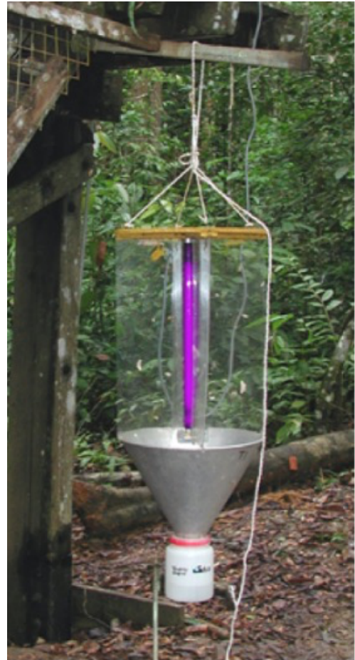
Fig. 1 Light trap set up at the canopy plot in Lambir Hills National Park. This trap is equipped with a rain shelter roof, a UV fluorescent lamp, four transparent acrylic plates for flying insects to collide and fall, a metal funnel, and a plastic container with chemicals to kill and preserve insects. This type of light trap was used in studies such as Kato et al. (1995, 2000), Itioka et al. (2001) and Kishimoto-Yamada et al. (2009). (Photo by Tamiji Inoue)
