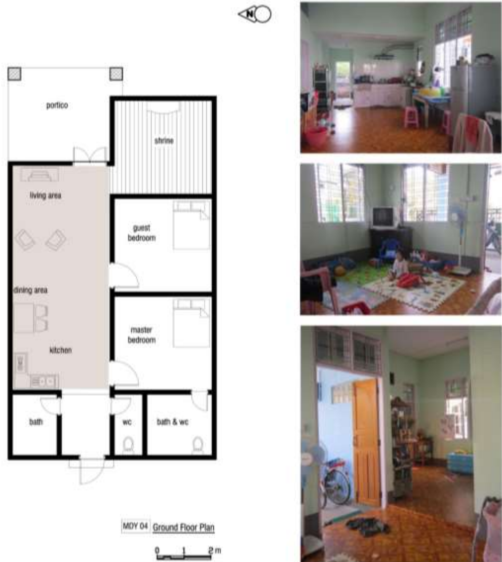
Figure 4.8. Single storey RCC building in Mandalay (Completion in 2015)
