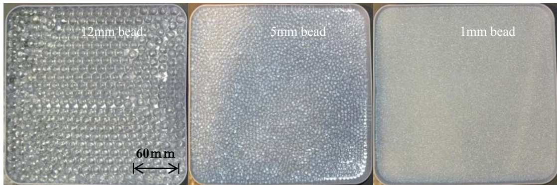
Figure 2.1: Solid matrix of spherical glass beads
