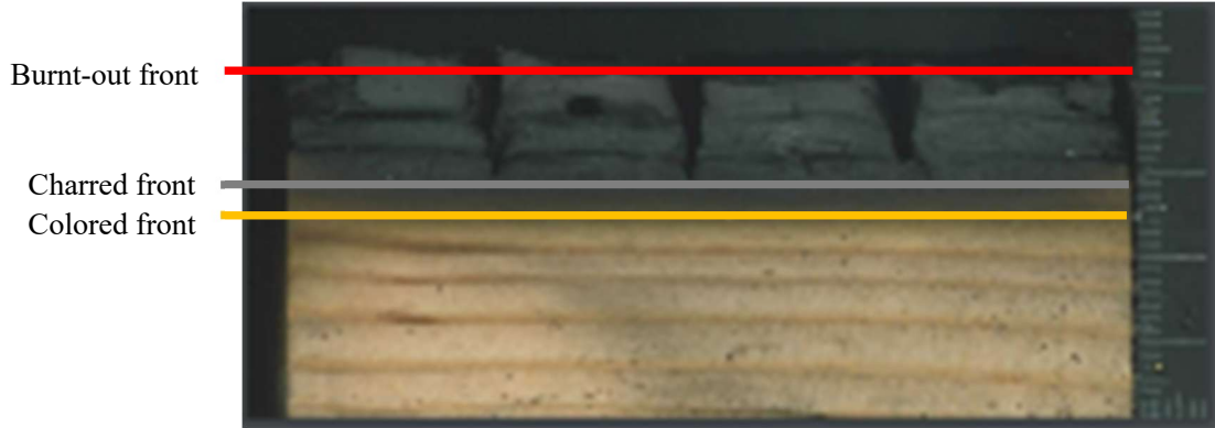
Figure 10: Example of location of colored, charred, brittle charred and burnt-out front (S-30-2)
