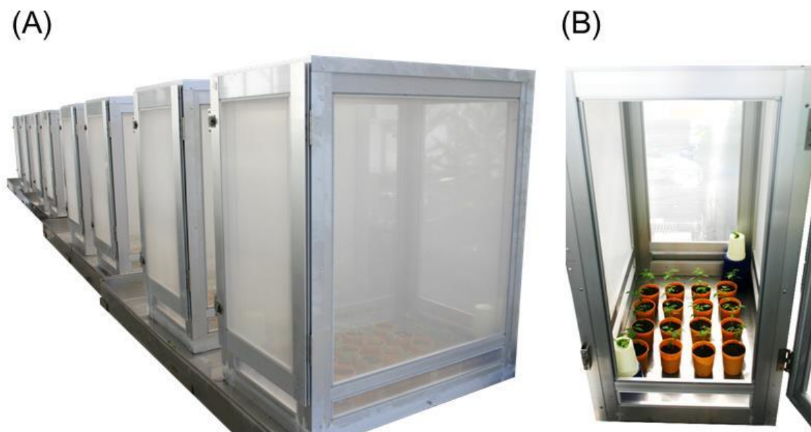
Fig. 6-1 Small aluminum chamber (69 cm in length, 44 cm in width, and 82 cm in height) for TYLCV transmission tests. (A) Whole picture of chambers, (B) Arrangement of potted grape tomato seedlings and inoculation source of adult whiteflies.
