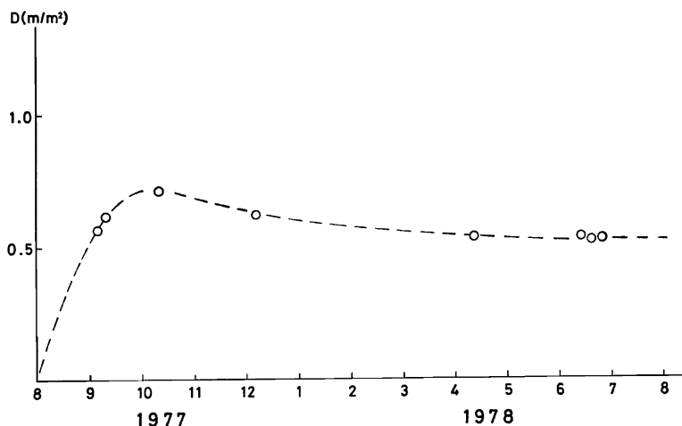
Fig. 2 The temporal change of the drainage density in the experimental slope (cf. Kashiwaya, 1980)
