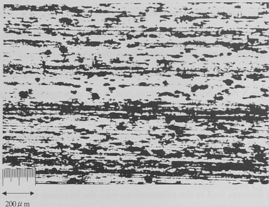
Figure 15: Optical micrograph of the counterface surface after wear test against the non-compressed sample
