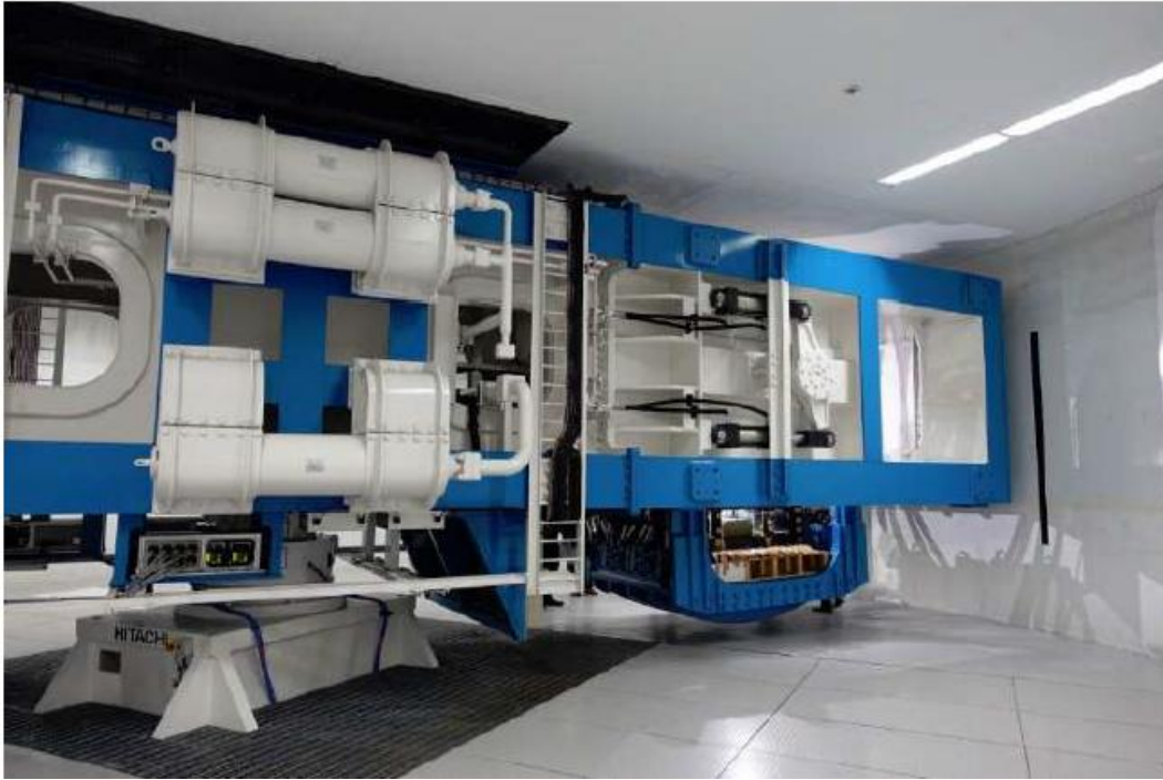
Figure 2.17. Large dynamic centrifuge loading equipment (Nanazawa et al., 2022).
