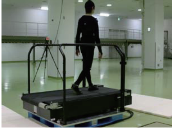
Fig. 3.3: Measurement of human splitbelt treadmill walking
