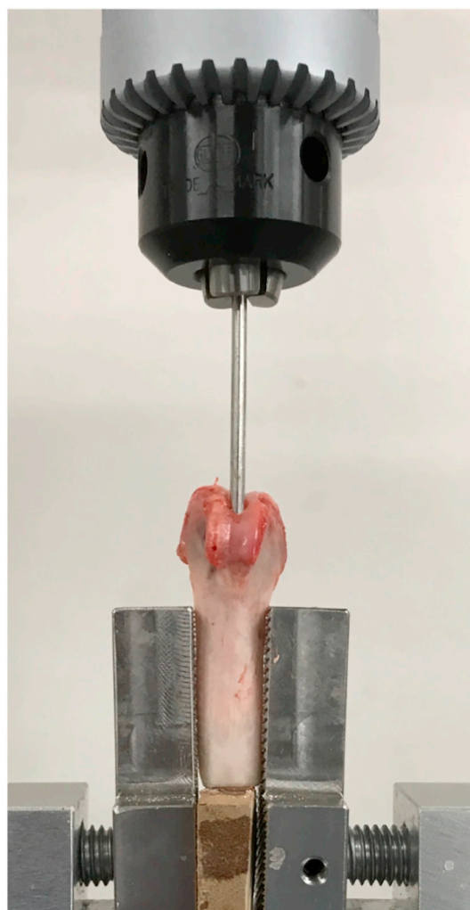
Fig. 1. Photograph of the push-out test. A femoral diaphyseal specimen with a composite rod as an intramedullary nail was gripped in the testing machine and pushed out by a Kirschner wire with a 2.0-mm diameter, at a crosshead speed of 20 mm/min.
