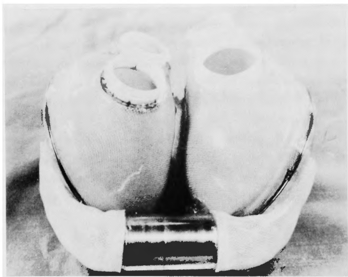
Fig. 38 Electrohydraulic hearts. Recently, a small, reversing, axial flow pump is utilized in the artificial heart. The mock circulation testing has demonstrated the function of these electrohydraulic hearts.
