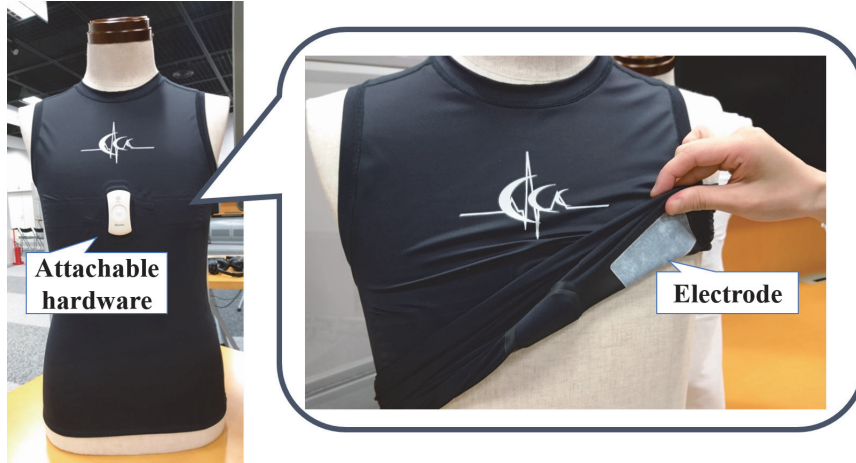
Figure 19: Example of easy-to-use T-shirt-type wearable device for unaided ECG measurement by non-experts (hitoe® [96]). Note that it additionally require a smartphone to receive and record signals transmitted from attachable hardware.
