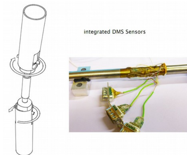
Fig.1: top: fixation of the protector to the body left: mechanism to limit combined 3D-movements; right: Strain gauge arrangement to measure torques in the horizontal, medial and frontal plane.
