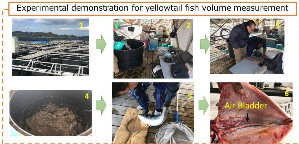
Fig. 6.6. Experimental demonstration for yellow tail fish volume measurement. Where: 1 is the cages where yellow tail fish are kept. 2 shows filling up of the 1000 L tank half with sea water. 3 experimental measurement in progress. 4 shows the fish with less movement in the water thus enabling measurement. 5 the fish was killed by stabbing and swim bladder was observed in 6.
