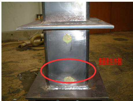
Photo 5.5 Damage of base of column (Pseudo-dyna test, X component)
