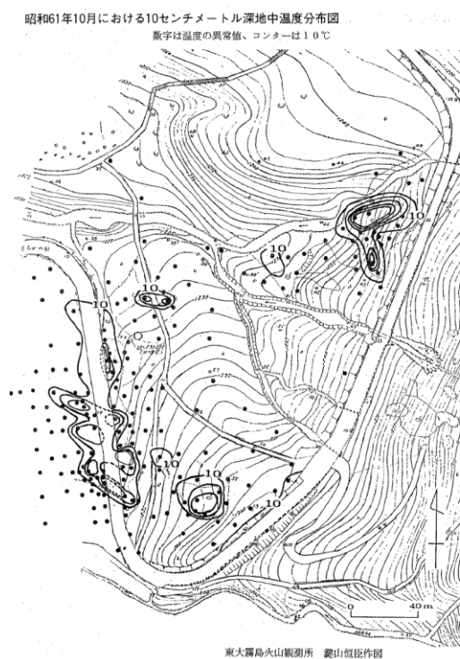
Fig. 13 Distribution of ground temperature at 10cm depth in 1986.
