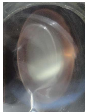
Fig. 2. Solid hydrogen in the target cell
