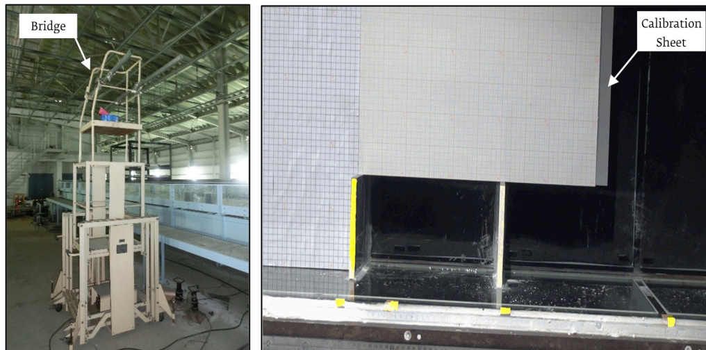
Figure 3-5. (Left) A view Bridge constructed over the flume to mount the camera; (Right) scaled sheet used for calibration of recorded images.
