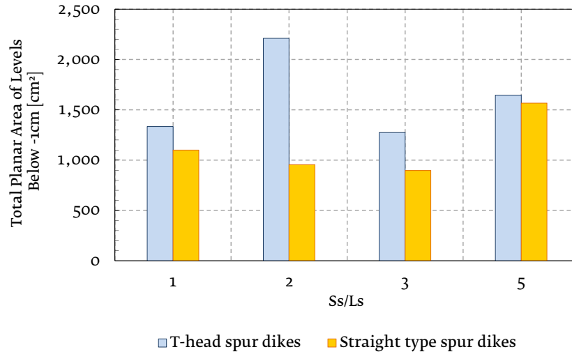
Figure 4-25. The planar area of scour zones below level “-1” cm in T-head and straight type spur dikes with different opening ratios ( Ss/Ls ), based on experimental data
