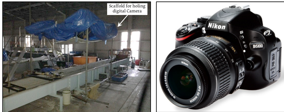
Figure 4-10. The scaffold mounted for holding the digital cameras (right photo) which were used for monitoring bed form migration
