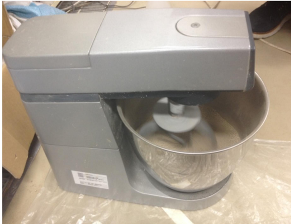
(a) Mixing under optimum water content
