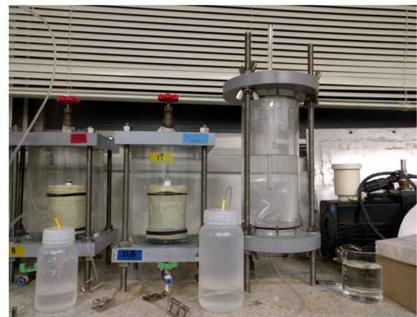
(f) Setting up of flexible-wall permeameter
