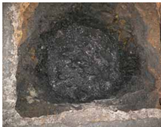
Photo 2 Hard rock in a hole excavated for setting the short span strainmeter.
