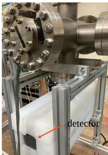
Fig. 2 The ^3\text{He} gas-filled detector under the chamber. Lead sheets and polyethylene blocks surrounded the detector.
