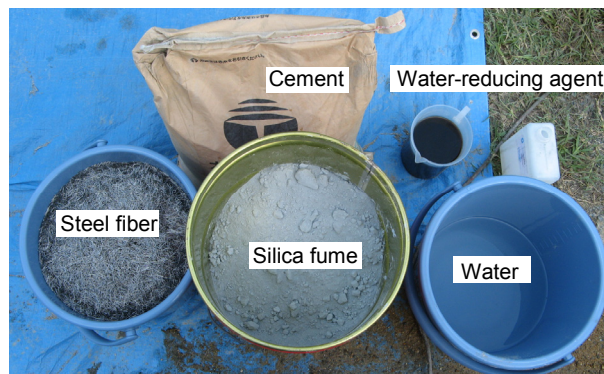
Fig. 4. 9 Mixing components of SFRCC
