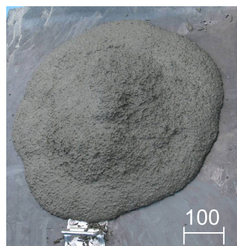
Fig. 4. 10 Slump test of SFRCC (unit: mm)
