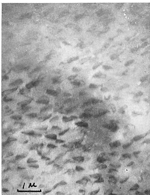
Photo. 21. Mg-11.6%Al alloy, W.Q., aged for 3.5 hr at 150°C. ( \times 10,000 )
