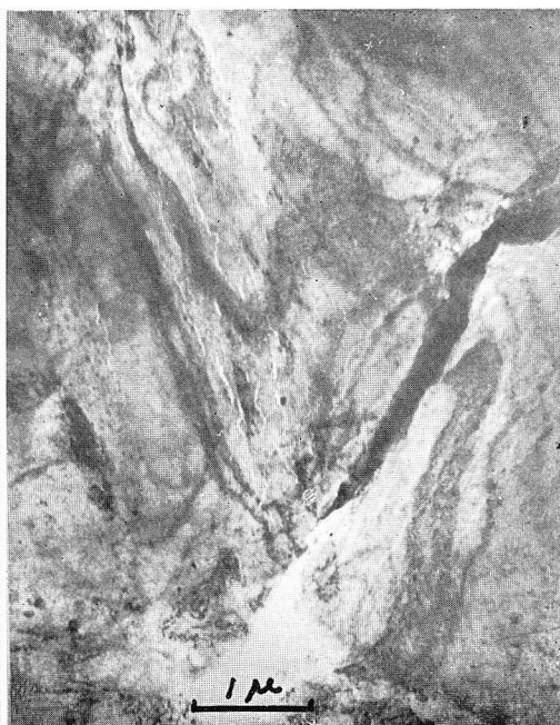
Photo. 23. Mg-11.6%Al alloy, W.Q., 60% roll ed, aged for 3 hr at 70°C. (14,000)
