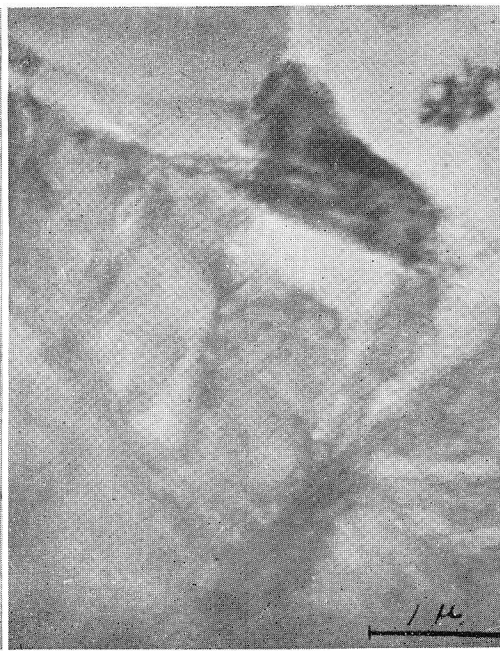
Photo. 3. Pure Mg, W.Q., 30% rolled, aged for 2 days at 70^\circ\text{C} ( \times 18,000 )
