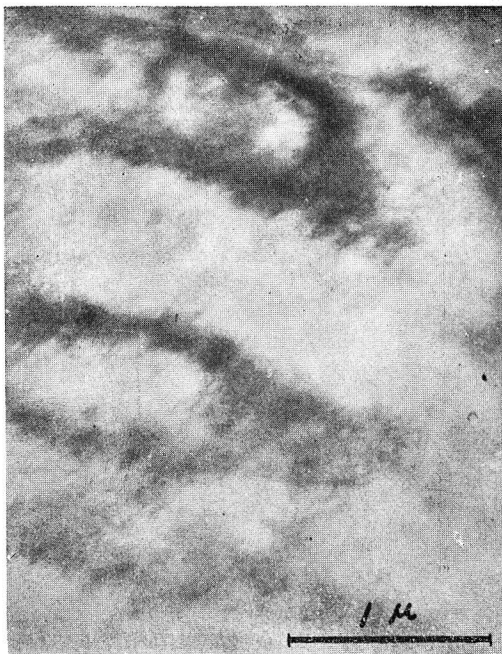
Photo 8. Mg-3.2%Zn alloy, W.Q., 30% rolled, aged for 5 days at 70°C. ( \times 27,000 )
