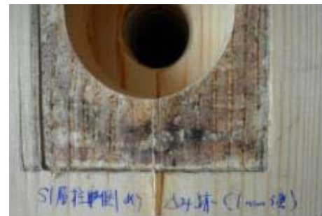
Figure 19 Permanent embedment deformation on the column side surface due to cyclic contact of steel box.
