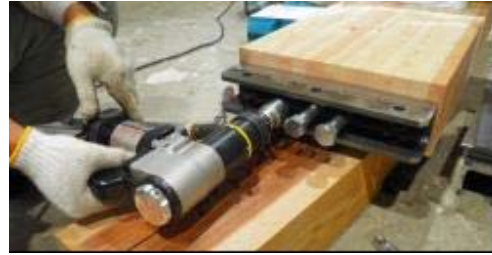
(a) Penetrating lag-screws for shear (previous experiments)
