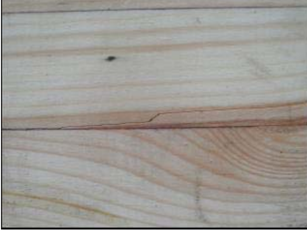
Figure 15 Small scale panel shear failure at the 1 st storey column-beam joint (photo was taken after all test was finished so glulam was laid horizontally).
