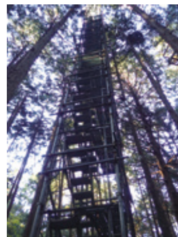
Flux measurement tower 30 m high
