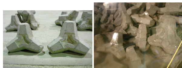
Photo 1 Wave absorbing block model
