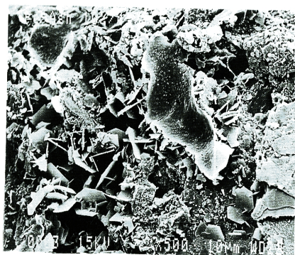
Photo 3 SEM of soil stabilized with 10% of Fe-Ash Lime after 28 days
