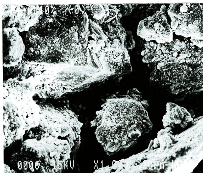
Photo 2 SEM of soil stabilized with 10% of Fe-Al Lime after 0 days
