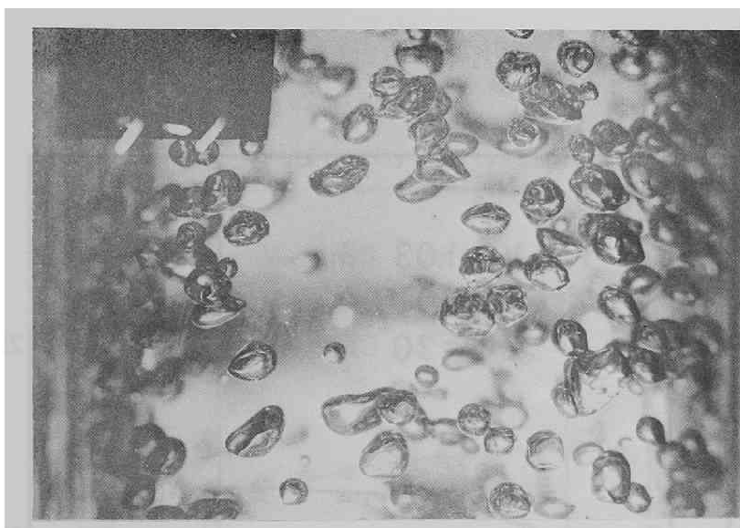
(a) Bubble flow (V_o = 1.03 \text{ m/sec}, X = 0.0085 \%, Z/D = 22.5)
