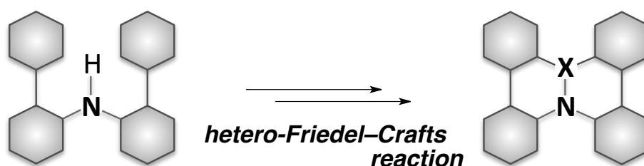
Scheme 1. Tandem hetero-Friedel–Crafts reaction producing a \pi -conjugated framework with a heteroatom junction
