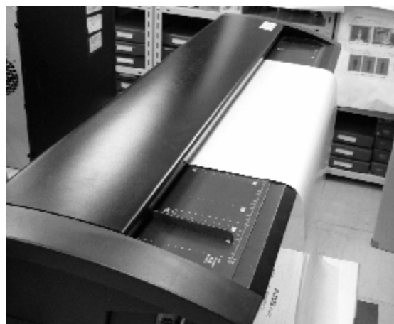
Fig. 3 Image scanner that can scan A0 size (CS2000 image scanner: GRAPHTEC.)
