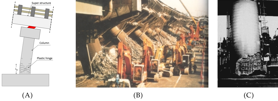
FIGURE 1.1: Illustration of: (A) the formation of plastic hinge in the conventional pier, (B) the bridge collapse [33], and (C) residual deformation of the pier due to Kobe earthquake in 1995 [17].
