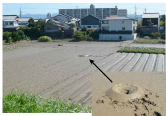
Photo 2 Sand volcano back of left bank of the Kamo river
