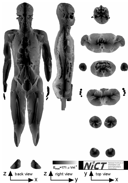
Figure 4. Electric field distributions and layer-maximum, layer-averaged, tissue-maximum, and tissue-averaged electric field strength ( \mu\text{Vm}^{-1} ) induced by 1 \mu\text{T} (peak), 50Hz, uniform B_k (foot-to-head) magnetic fields
