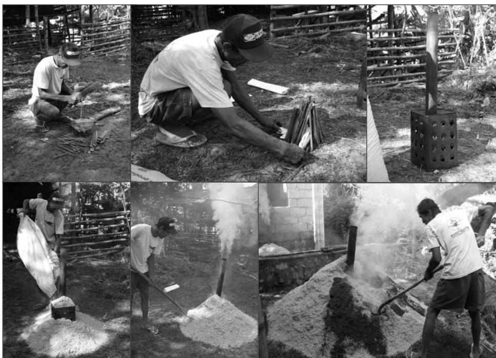
Fig. 5 Process of carbonizing rice hull. From top left: cutting small twigs as fuel and starting the fire; a hand-built carbonizer; pouring sacks of crude rice hull around the carbonizer; turning over the rice hull heap to ensure even heat distribution
