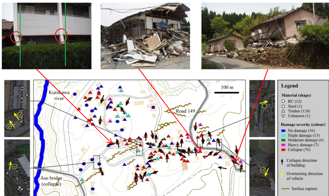
Figure 2-15 Field survey on damage of buildings, collapse of vehicles (the collapse of vehicles was surveyed by Google Earth)
