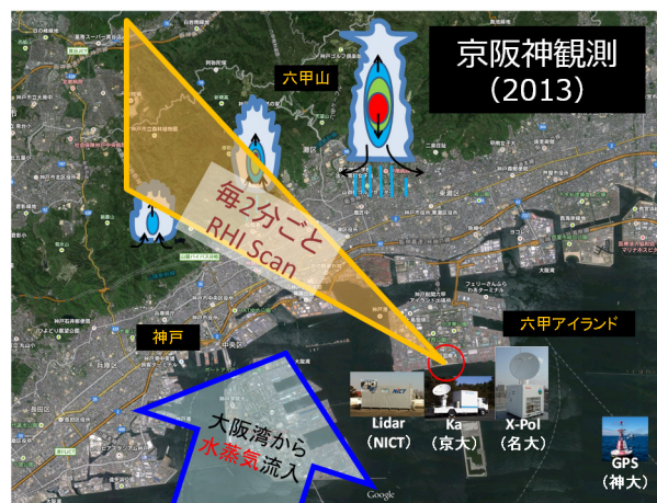
Figure 2 RHI scanning with every 2 minutes using multi-sensors
