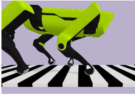
Figure A.2: A screen shot of a preliminary experiment on surfaces with zebra-patterned bands. The white bands have a lower friction coefficient than the black bands.
