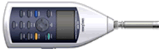
Fig.2.12 Noise meter ( www.onosokki.co.jp/English/hp_e/products )
