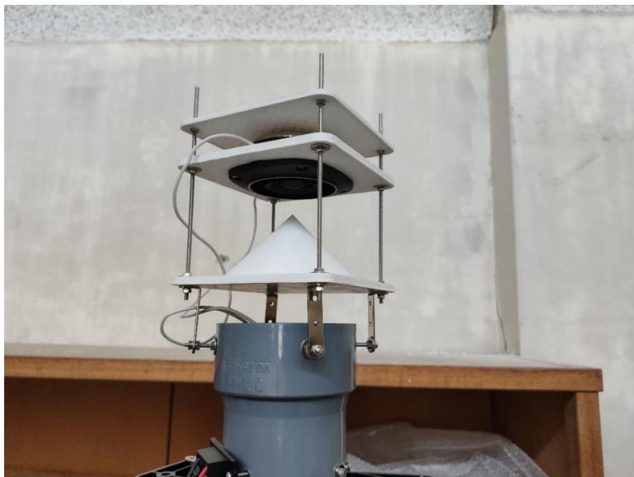
Fig.2.8 Speaker with cone
