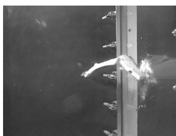
Photo 2 Instantaneous pictures of roof tile impact recorded by high-speed video camera
