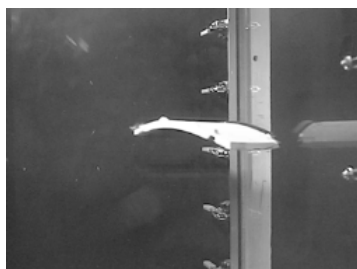
Photo 2 Instantaneous pictures of roof tile impact recorded by high-speed video camera
