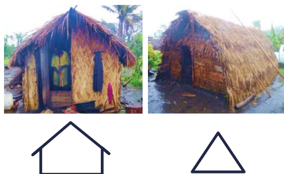
Figure 7. Local house (left top) and Nimulaten (right top) and geometric characteristics of their vertical cross sections (bottom).
