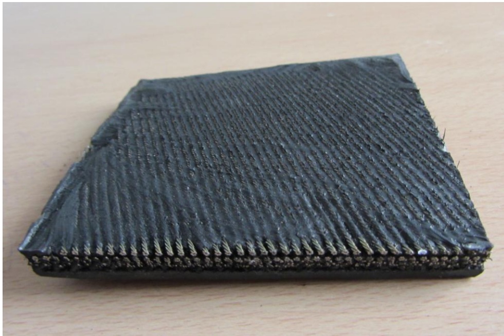
Figure 3.1 Photograph of single layer STRP showing layout of steel reinforcing cords
