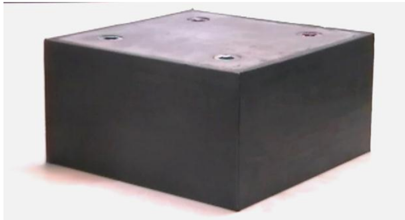
Figure 2.8 1/4 scale fiber reinforced elastomeric isolator
