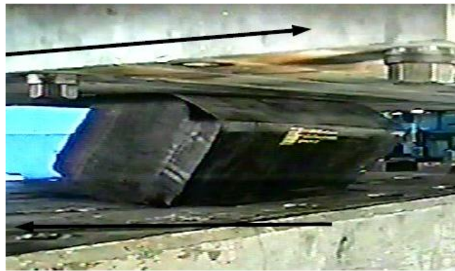
Figure 2.1 Steel laminated elastomeric bearing without fastening system
