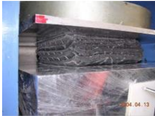
Figure 2.9 Test setup with scrap tire pads
