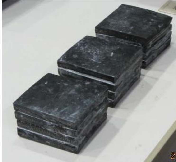
Figure 6.4 Photograph of layer-bonded STRP-4 specimen bearings
