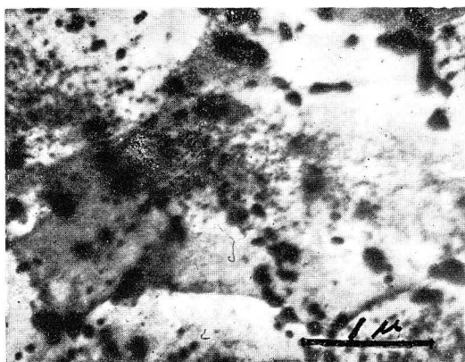
Photo. 32. Mg-5.6%Zn alloy, W.Q., 40% rolled, aged for 13 days at 150°C. ( \times 20000 )
