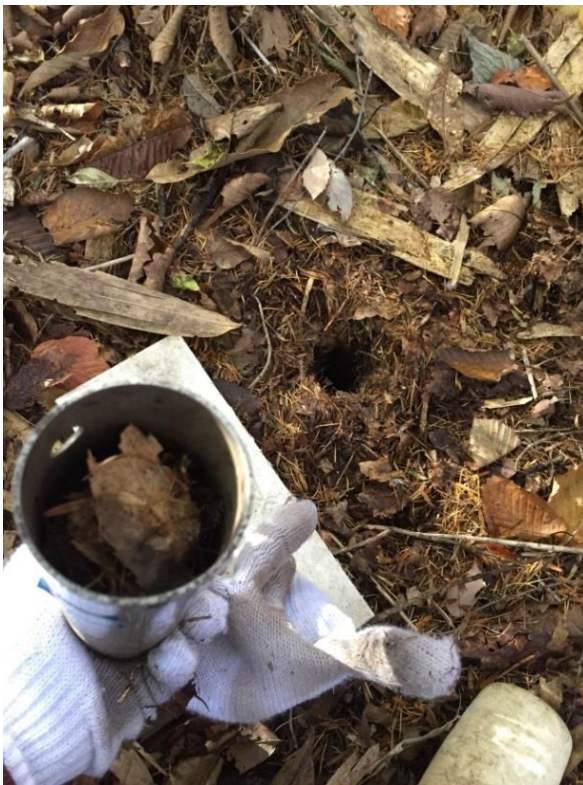
Figure 5.6 Core sampling by the auger and the section description of one example soil layer
