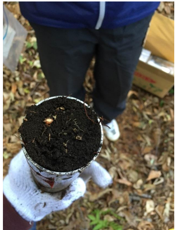
Figure 5.6 Core sampling by the auger and the section description of one example soil layer
