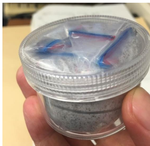
Figure 5.8 The soil sample and the plastic bag were put in the plastic box before the detection of the radioactivity
